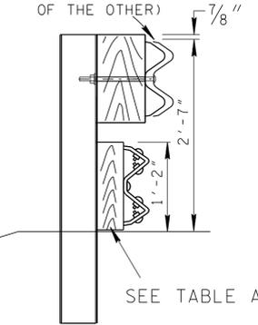
12'-6" UPPER SECTION OF W-BEAM GUARDRAIL WHICH IS TO BE NESTED (TWO SECTIONS THICK WITH ONE SECTION IN FRONT OF THE OTHER)
