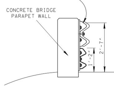
12'-6" UPPER SECTION OF W-BEAM GUARDRAIL WHICH IS TO BE NESTED (TWO SECTIONS THICK WITH ONE SECTION IN FRONT OF THE OTHER)
